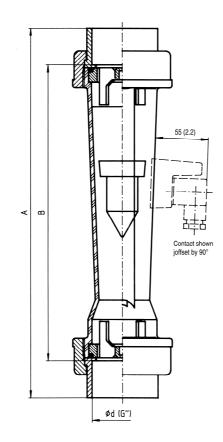
Fig. 4 FVA Trogflux short version, dimensions in mm
