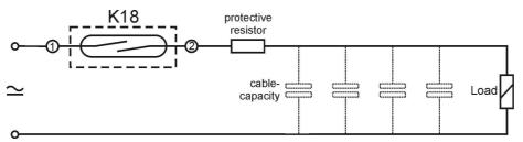
Fig.7 Protective circuit for current limitation
