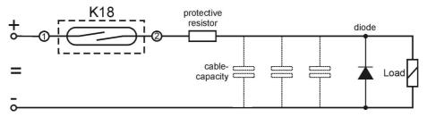
Fig.8 Protective circuit for inductive loads and DC power supply
